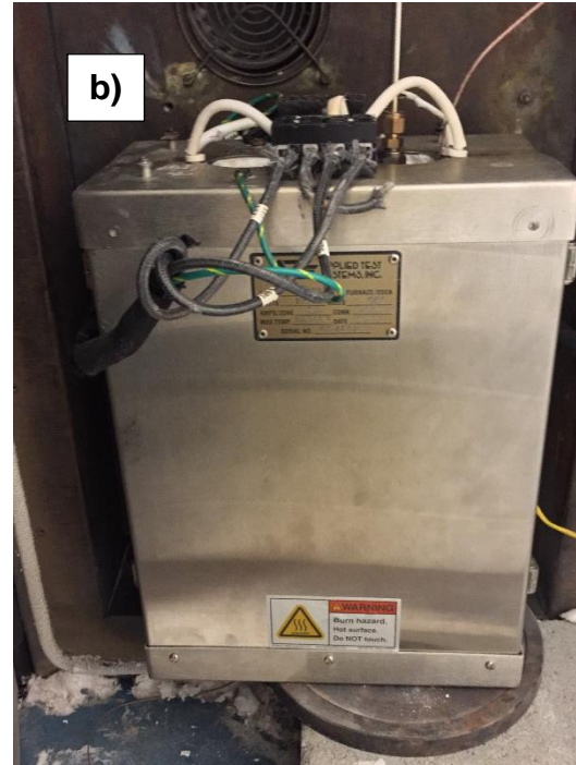
Figure 3.9. a) Image captured by webcam during a sample rupture and b) Furnace used for burst test.
