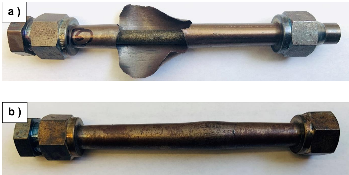
Figure 5.23. Typical burst test specimens (a) direct open-up, (b) small crack and hole opening.
