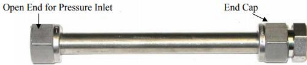
Figure 3.7. FeCrAl sample used for burst testing.
