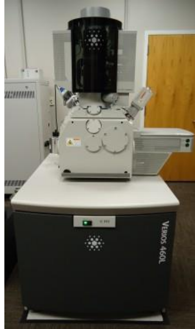
Figure 3.6. VERIOS SEM equipped with EBSD at AIF.
